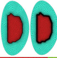
Left image is a layered mesh with 5 elements through wall. Mesh has 4.9K elements. Right image is an isotropic mesh with mesh sizes set to get similar through thickness resolution. Mesh has 19K elements (4 times more).
