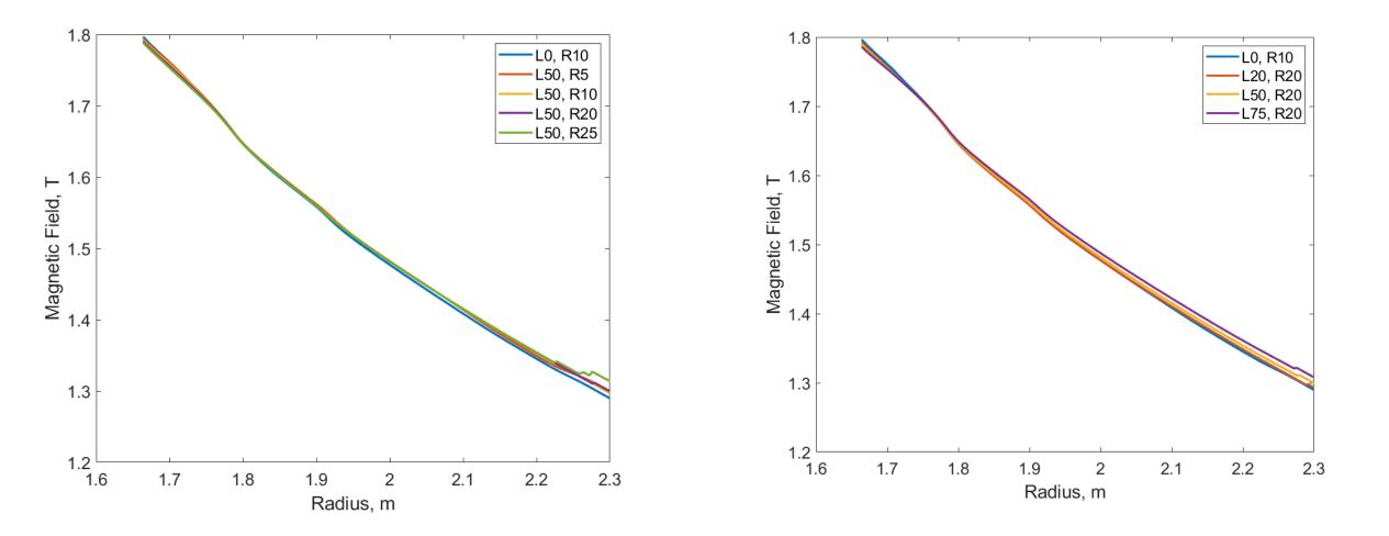
• Magnetic field is neither sensitive to the disk radius nor to the longitudinal displacements
