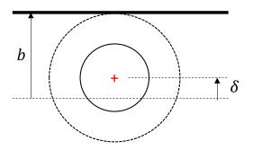
Wall current is calculated with the image method. DOES NOT consider CQ induction!
