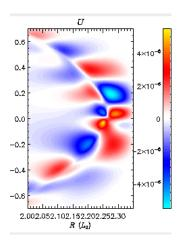
Density perturbation causes decreased Te at one location on flux surface. Thermal conduction during linear phase causes pressure to increase there. Gives an unstable mode for ntor=9 only if kappar .ne. 0
