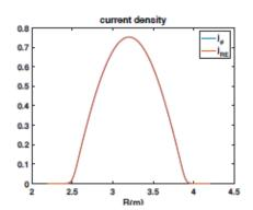
$$\begin{array}{ll} \bullet & {\sf Parameters:} & \beta_0 = 0.15 \\ & a = 0.65m \\ & {\sf R} = 1.7m \\ & B_0 = 1.9T \\ & \eta = 1.0 {\times} 10^{-4} \\ & n_0 = 1.0 {\times} 10^{20} m^{-3} \\ & c = 150 v_A \\ & N_{elements} = 12261 \\ & \Delta t = 1.0 \tau_4 \end{array}$$
