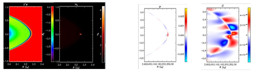
Density perturbation causes decreased Te at one location on flux surface. Thermal conduction during linear phase causes pressure to increase there. Gives an unstable mode for ntor=9 only if kappar .ne. 0
