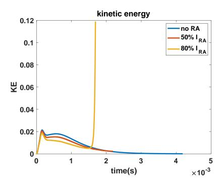
The case with 80% runaway current has instability at about t=1.5ms. No runaway current and 50% runaway current cases do not have instabilities.
